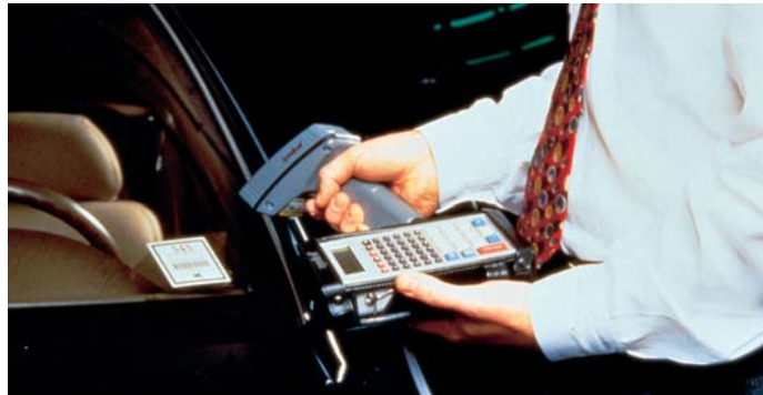
An APCOA/Standard Parking employee uses a computer and scanning gun to inventory a vehicle via its bar code.
